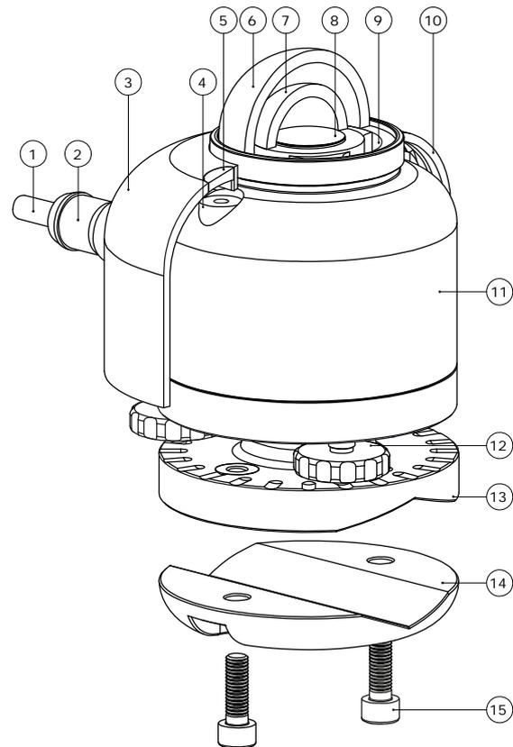
**Figure 7** overview of SR30: (1) cable, (2) connector, (3) sun screen, (4) bubble level, (5) bubble level window, (6) outer dome, (7) inner dome, (8) thermal sensor with black coating, (9) internal ventilation vents, (10) quick release system of sun screen, (11) instrument body, (12) levelling feet, (13) optional spring-loaded levelling mount, (14) optional tube mount, (15) screws included with tube mount
